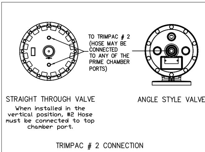
Figure 11 - Valve Connections
