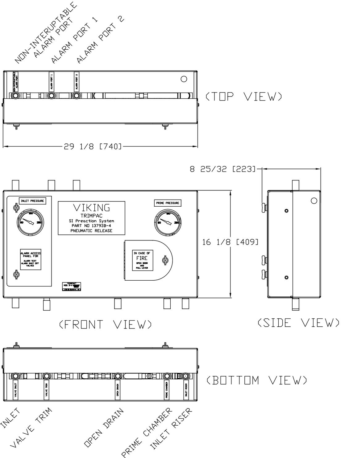
**Figure 2 - TRIMPAC® Model B-4, B-4B & B-4S Dimensions**
